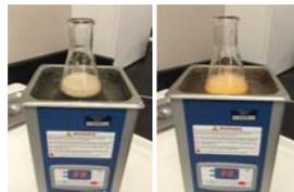
Figure 2: Degassing of Reef cola (left) and Orange kush (right)
