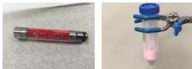
Figure 1: Hard candy before (left) and after (right) freezer mill grinding
